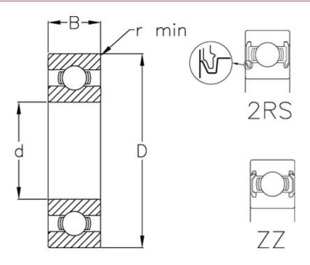
B = 5 d = 15 D = 24 Dynamic load C (kN) = 2.08 Max rpm greased = 26000 Max rpm oil lubricated = 31000 r min = 0.3 Static load C0 (kN) = 1.26
